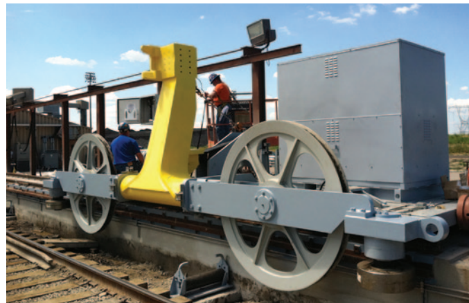
130 Car Positioner - Wire Rope Drive – up to 300,000 lbs (1,334 kN) pulling capacity.
