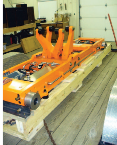
30 Car Positioner – Hydraulically Driven – Travels in between the track rails beneath the railcars.
