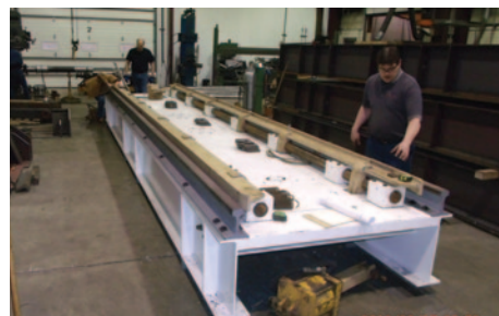
Retarders – Air operated. Generous mis-spotting capability. Holding capacities up to 20,000 lbs (89 kN).
