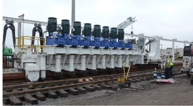
160 Car Positioner - Rack & Pinion Drive – up to 400,000 lbs (1,800 kN) pulling capacity. Largest in the USA.
