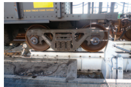
Model 100 Truck Locks – 100,000 lbs (445 kN) holding capacity – Hydraulically activated.
