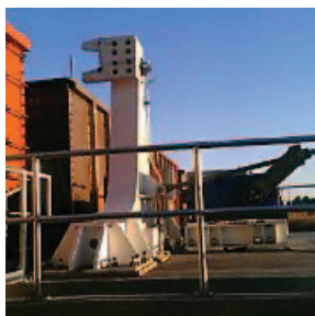
Holding Arm – 150,000 lbs (667 kN) holding capacity – Mechanically Operated.
