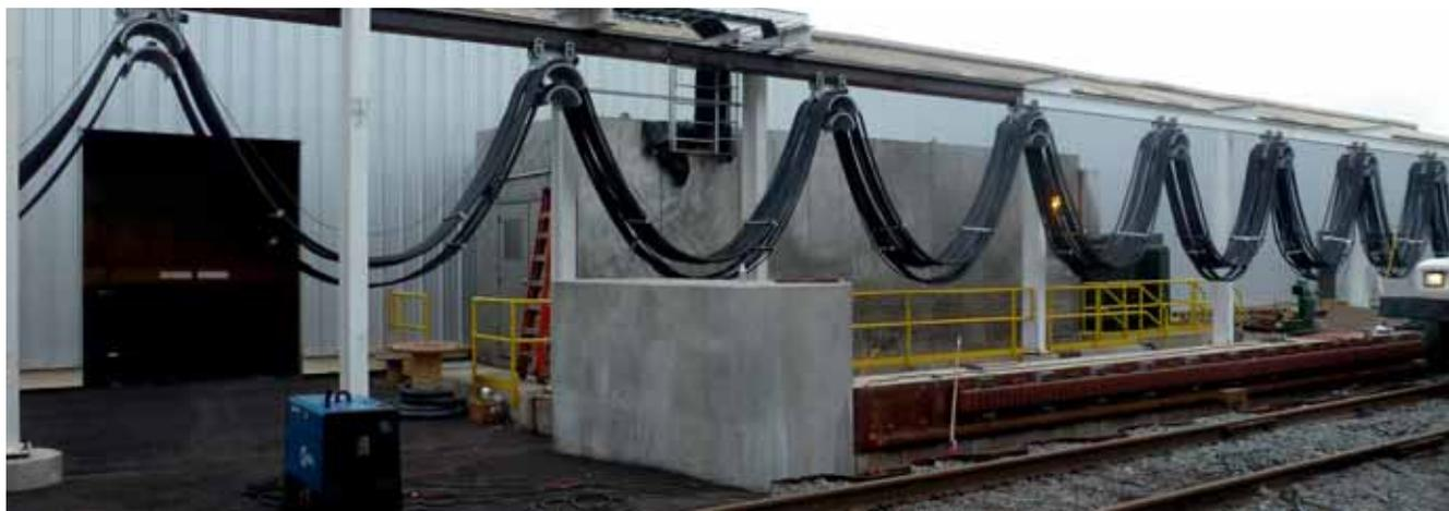
340ft, with a loop depth of 10.50ft, and cable weight per loop of 650 pounds.”
